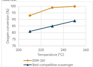
An increase of the contact time to about two seconds allows 100% conversion of oxygen to be reached for this whole temperature range.
