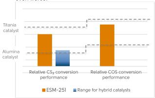
The ESM-251 is radically different. It employs a proprietary promoter to achieve a  $CS_2$  conversion performance that is significantly higher than that of an alumina catalyst. The COS conversion performance is even more remarkable, and comes close to that of a titania catalyst.
