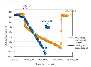
Alumina based catalyst are not as easily revived; they first need to be fully oxidised again. Fully oxidising the catalyst is very risky due to the possible sintering of the CoMo metals, which could lead to irreversible deactivation of the catalyst. Additionally, during both the oxidation and presulphiding the sulphur emissions will be much higher than usual. These issues are a problem of the past when using our ESM-281 titania based TGT catalyst.
