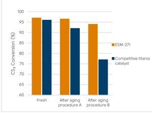
Although the performance level of the fresh catalysts is quite similar, the ESM-271 shows a significant advantage as aged catalyst. This is especially apparent after the more severe aging of procedure B. Pure titania catalysts remain active even after severe aging.
